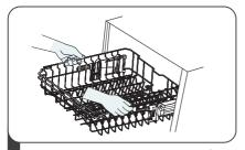
To raise the upper basket, just lift the upper basket at the center of each side until the basket locks into place in the upper position. It is not necessary to lift the adjuster handle.
