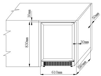
• Please provide a minimum of 30mm on the top and sides and 50mm at the back of the wine cellar Note: Leave an additional 15mm gap for access to door handle if installed in a niche
