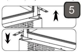
6. Locate the glass door to the designated position making sure that the door shaft enters the door hole at the left upper corner of the glass door. Install the two screws that are used to connect the lower hinge with the glass door and tighten them before the door is leveled.
