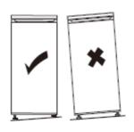
If the appliance is not level, the doors will not be correctly aligned and the compartment seal cannot be guaranteed.
