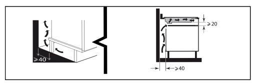
or above a built-in oven, comply with the dimensions provided on the illustrations to ensure a sufficient air outlet at the front.
