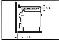
Carefully glue the sealing joint to the entire surround of the glass hob and insert the table into the cabinet.
