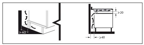
or above a built-in oven, comply with the dimensions provided on the illustrations to ensure a sufficient air outlet at the front.
