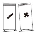
If the appliance is not level, the doors will not be correctly aligned and the compartment seal cannot be guaranteed.
