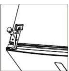
10. Take left hinge cover from accessary bag and install it with top hinge. Then install hole cover at right side.
