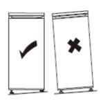
If the appliance is not level, the doors will not be correctly aligned and compartment sealing will not be ensured.
