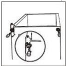
7. Unscrew right middle stopper with metal block from bottom of upper door. Then install left middle stopper and metal block in left side of bottom of upper door. (The same operation as for lower door.).
