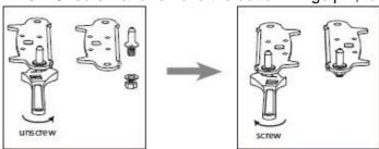
6. Refit the bracket fitting the bottom hinge pin. Replace both adjustable feet. Transfer the lower door to the property position.
