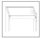
10. Unscrew and remove the bottom hinge pin, turn the bracket over and replace it.
