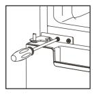
15.Replace upper door, please ensure the door align with the cabinet to make sure door gasket seal the cabinet tightly. Then connect door with cabinet by tightly fixed top hinge.
