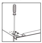
16.Connect harnesses from door and cabinet. Then replace top hinge cover. Before screw the cover, connect terminals of door switch.
