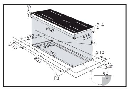
Flush fitting installation
